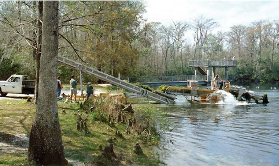
Mechanical harvester at work (Photo by Jeff Schardt, UF/IFAS/CAIP; used with permission)
