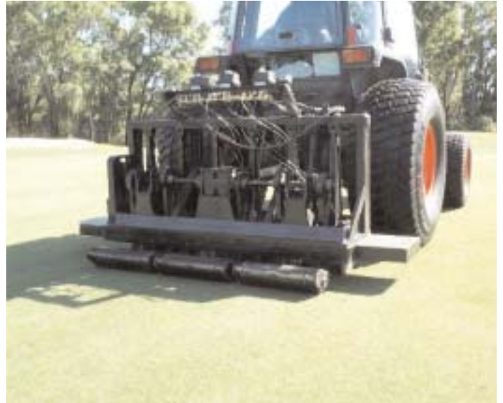
Figure 8 Application equipment injecting 1,3-dichloropropene into a putting green
